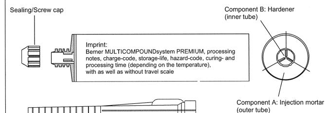
Static Mixer, one-way tool, must be changed in case of working interruption
