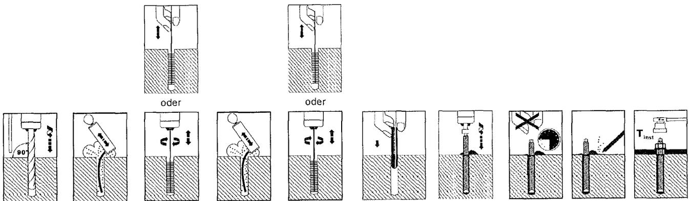
Würth Verbundanker W-VD/S, W-VD/F, W-VD/A4, W-VD/HCR
