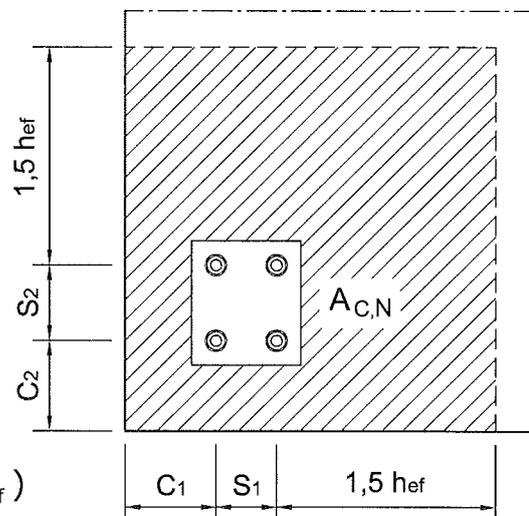
$$A_{C,N} = (c_1 + s_1 + 1,5h_{ef}) \cdot (c_2 + s_2 + 1,5h_{ef})$$
