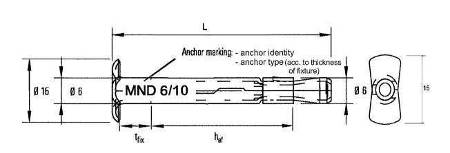
Table 1: Anchor dimension, marking and material
