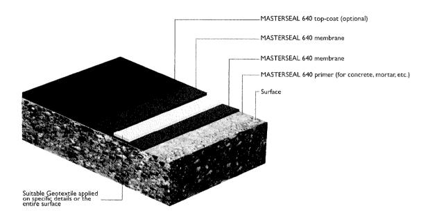
Applicable to the roof waterproofing "MASTERSEAL 640 membrane":
