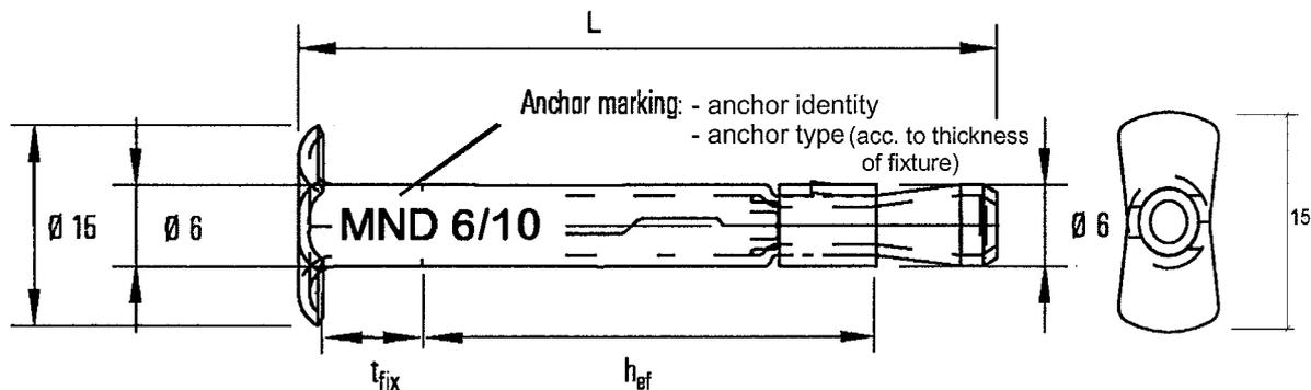
**Table 1:** Anchor dimension, marking and material
