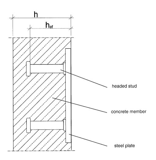
h<sub>ef</sub> = effective anchorage depth h = thickness of concrete member
