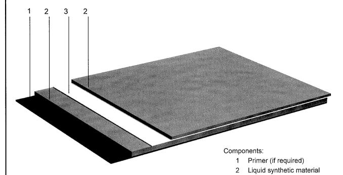
Applicable to the roof waterproofing "Icopal-PROFI-DICHT":
