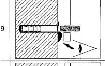
Check if excess mortar seeps from the hole. If the hole is not completely filled, pull out anchor rod, let mortar cure, drill out hole and start again from No. 2.
