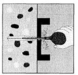
Removal of drill dust e.g. blowing
