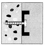
Complete verification: head supported to fixture and embedment depth  $h_{nom}$
