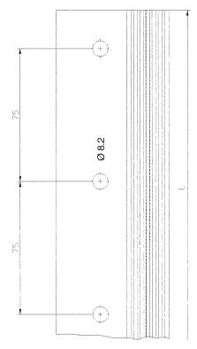
Vertical connection profile - "Grigolin Verbindungschiene" (dimensions in millimetres)
