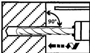
Drill hole perpendicular to concrete surface.
