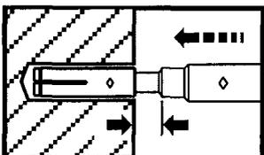
Drive in cone by using setting tool.
