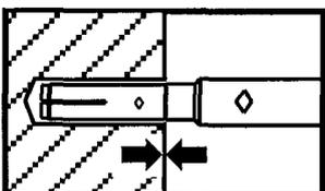
Shoulder of setting tool must fit on anchor rim.
