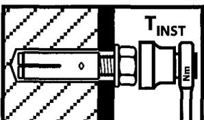
Apply installation torque  $T_{inst}$  by using torque wrench.
