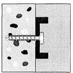
Complete verification: head supported to fixture and embedment depth h<sub>nom</sub>
