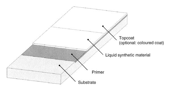
Applicable to the roof waterproofing "VEDASEAL":
