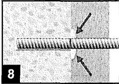
**8** Be sure that the bar is inserted in the bore hole until the embedment mark is at the concrete surface and that excess mortar is visible at the top of the hole. If these requirements are not maintained, the application has to be renewed.
