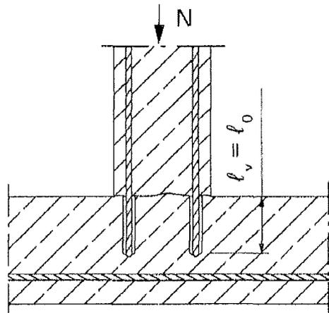
**Figure 5:** Anchoring of reinforcement to cover the line of acting tensile force
