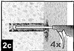
2c Finally blow the hole clean again with compressed air or a hand pump a minimum of four times. If the bore hole ground is not reached an extension shall be used.
