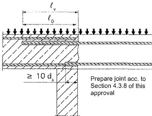
**Figure 2:** Overlapping joint at a foundation of a wall or column where the rebars are stressed in tension
