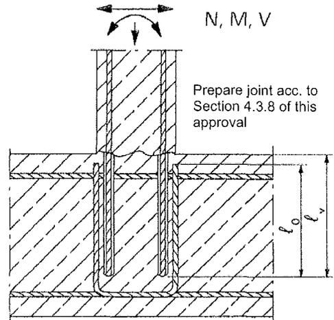
**Figure 3:** End anchoring of slabs or beams, designed as simply supported
