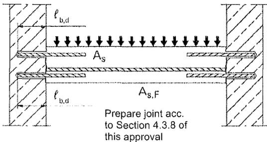
**Figure 4:** Rebar connection for components stressed primarily in compression. The rebars are stressed in compression
