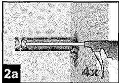
2a Starting from the bottom or back of the bore hole, blow the hole clean with compressed air or a hand pump a minimum of four times. If the bore hole ground is not reached an extension shall be used.
