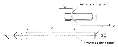
Marking: Works symbol / Length of threaded rod. or: Works symbol Property class 8.8 additional \*; Stainless steel additional A4; High corrosion-resistant steel additional C.
