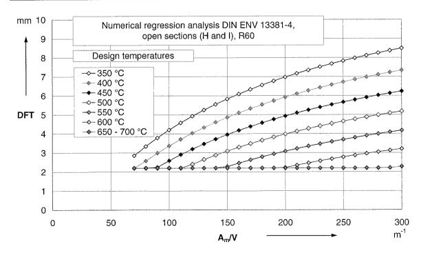
Annex 1, Table 4: Beams and columns, open sections (H und I)
