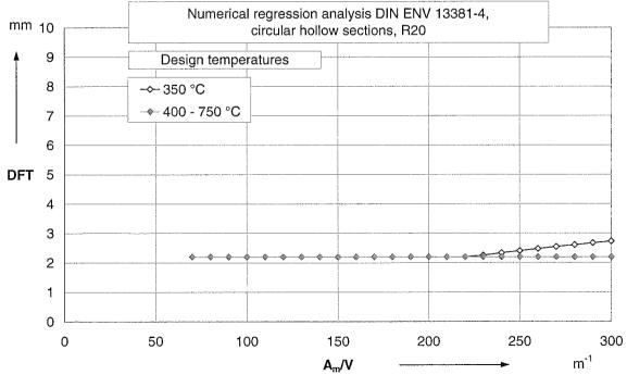
Annex 1, Table 15: Beams and columns, circular hollow sections
