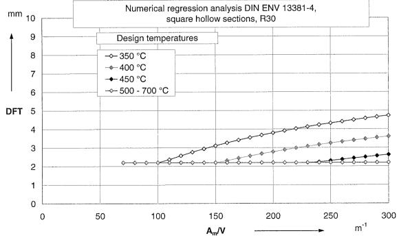
Annex 1, Table 9: Beams and columns, square hollow sections
