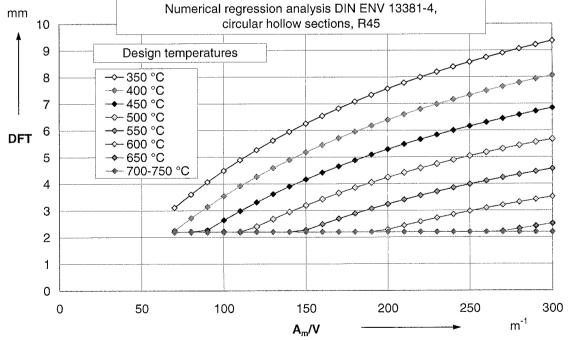
Annex 1, Table 17: Beams and columns, circular hollow sections
