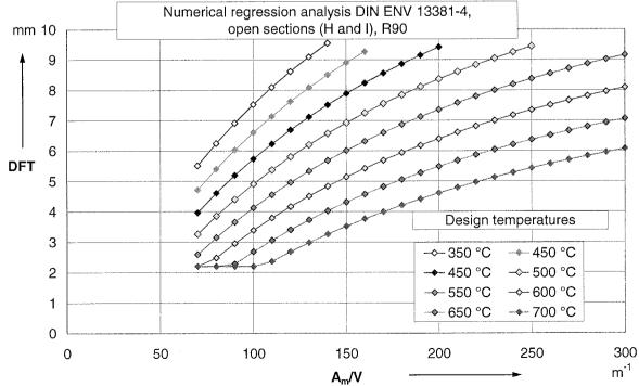
Annex 1, Table 5: Beams and columns, open sections (H und I)
