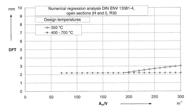
Annex 1, Table 2: Beams and columns, open sections (H und I)
