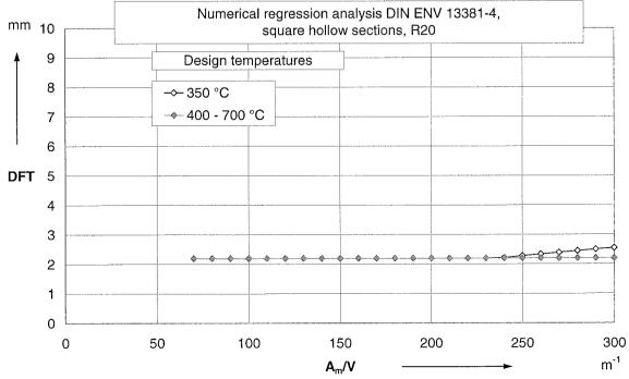
Annex 1, Table 8: Beams and columns, square hollow sections
