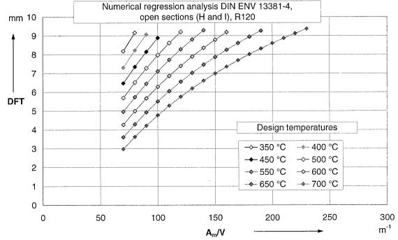
Annex 1, Table 6: Beams and columns, open sections (H und I)
