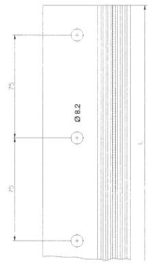
**Vertical connection profile – "Verbindungsleiste PVC"** (dimensions in millimetres)
