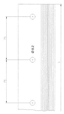
Vertical connection profile – "Verbindungsleiste PVC" (dimensions in millimetres)
