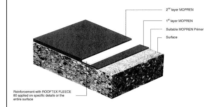
Applicable to the roof waterproofing "MOPREN SYSTEM":
