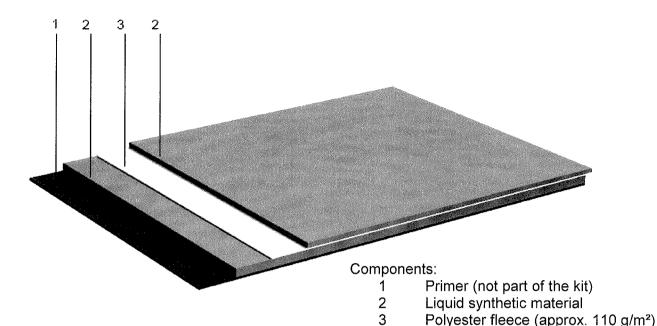
Applicable to the roof waterproofing system "Triflex ProThan" and "Triflex ProThan Detail":
