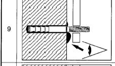
Check if excess mortar seeps from the hole. If the hole is not completely filled, pull out anchor rod, let mortar cure, drill out hole and start again from No. 2.
