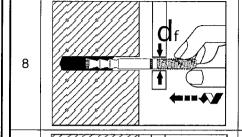
Insert the anchor rod VMZ-A by hand, rotating slightly up to the full embedment depth.
