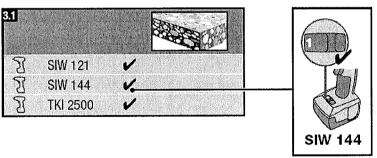
Hand setting of HUS-HR in concrete base material not allowed (machine setting only)
