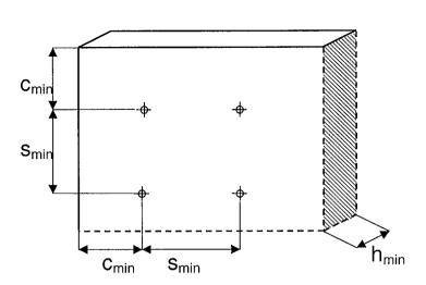
**Table 6:** Minimum thickness of concrete member, minimum spacing and minimum edge distances of anchors
