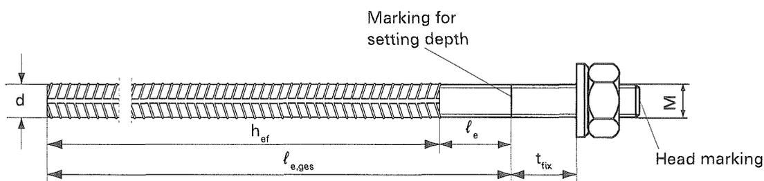
Head marking e.g.: FRA (for stainless steel); FRA C (for high corrosion-resistant steel)
