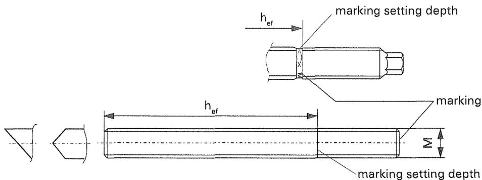
**Marking:** Works symbol / Length of threaded rod. or: Works symbol
