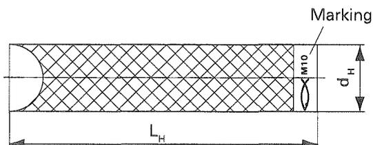
**Marking:** Works symbol and anchor size
