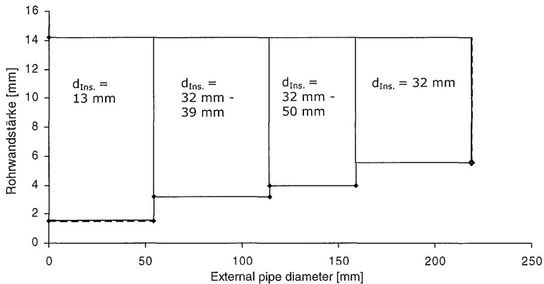
**Field of application for "PYROSTAT-UNI RM", "PYROSTAT-UNI RMB" and "PYROSTAT-UNI RM-LT"**
