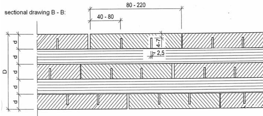
d = thickness of board ( $10 \text{ mm} \leq d \leq 33 \text{ mm}$ )
