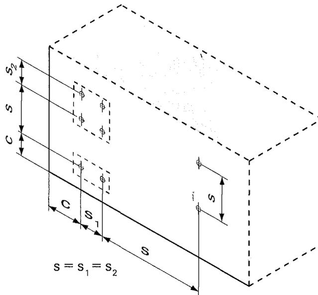
fischer injection system FIS V masonry
