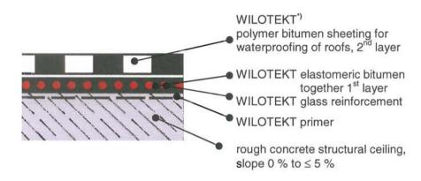
Instead of the WILOTEKT-polymer bitumen sheeting it can be used a CE marked polymer bitumen sheeting according to EN 13707 or EN 13969 which meet the specification stated in annex 2.
