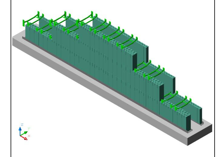
**QUAD-LOCK Building Solutions**Permanent Insulating Concrete Forms
