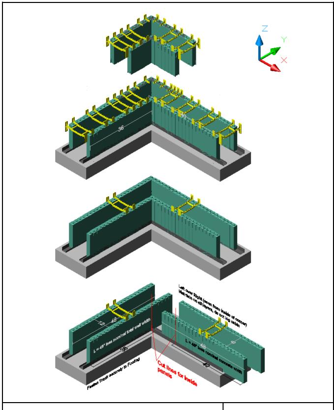
Construction of 90° Corners - Sequence Placement and Cutting of EPS Panels, Ties and Corner Brackets
