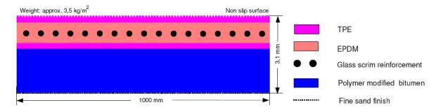
Bitumen - compatible, heat weld able, EPDM synthetic rubber membrane
