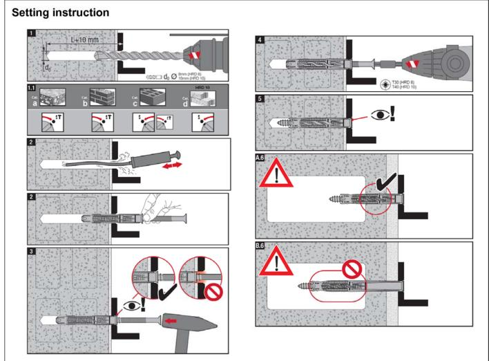
Additional preparation in case of application in precast prestressed hollow core slabs After drilling follow the main instruction above
