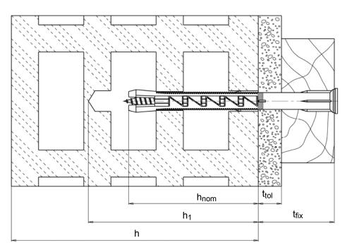
$h_{\text{nom}}$ : Overall plastic anchor embedment depth in the base material
