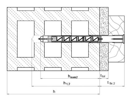
h<sub>nom1</sub>: Overall plastic anchor embedment depth in the base material (1)
