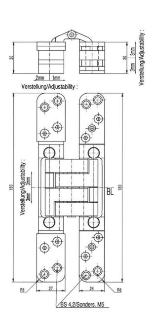
Variable concealed three part hinges PIVOTA ® DX 60 3-D
