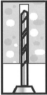
drilling of hole
