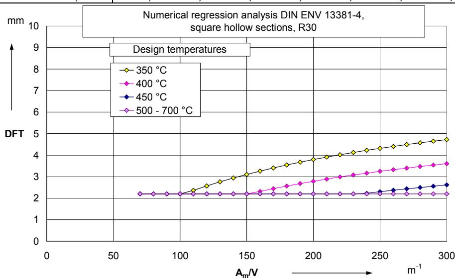
Annex 1, Table 11: Beams and columns, square hollow sections
