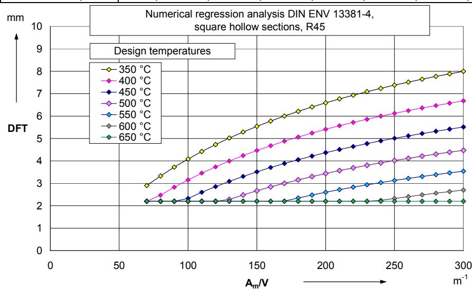
Annex 1, Table 12: Beams and columns, square hollow sections
