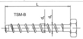
Anchor version with connection thread Designation e.g. TSM-BS6x100 M8x35
