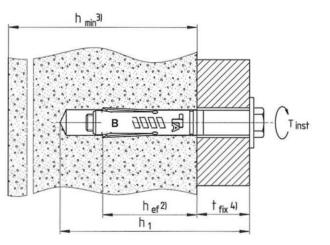
$^{1)}$  Length of hexagon head bolt  $L_{S}$   $^{2)}$  Effective anchorage depth  $h_{ef}$   $^{3)}$  Minimum thickness of concrete member  $h_{min}$   $^{4)}$  Thickness of fixture  $t_{fix}$
