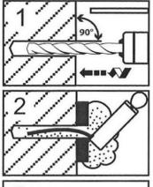
Drill hole perpendicular to concrete surface.
