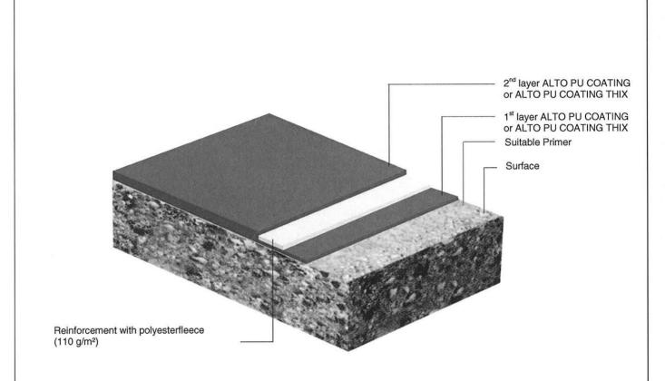
Applicable to the roof waterproofing "ALTO PU COATING" or "ALTO PU COATING THIX":
