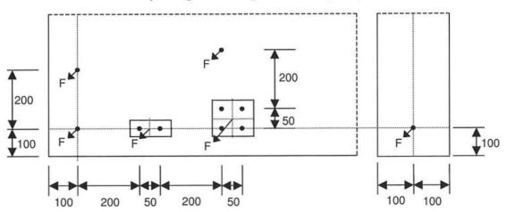
The characteristic values of resistance F<sub>Rk</sub> are valid for one fixing point. A fixing point can be:
