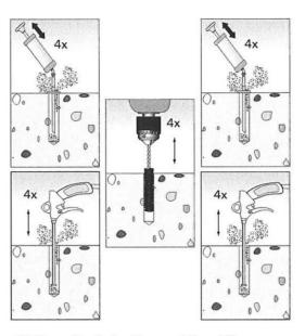
2) Clean the hole: Blow out the drill hole four times, brush four times and blow out four times again. For drill hole diameter ≥ 18 mm use oilfree pressure air (P > 6 bar).
