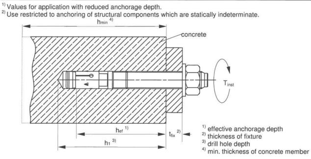
Minimum thickness of concrete members, minimum spacing and Table 4: minimum edge distances of anchors
