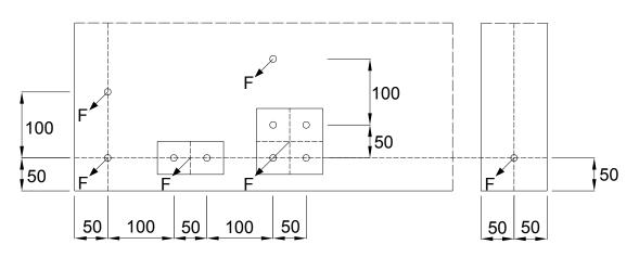
The characteristic resistance  $F_{Rk}$  applies to one fixing point. A fixing point can be:
