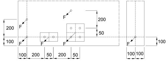
The characteristic resistance  $F_{Rk}$  applies to one fixing point. A fixing point can be:
