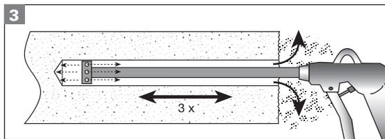
**Blowing out the drill hole (control)**
