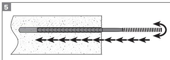
**The rebar may only be loaded after full curing!**
