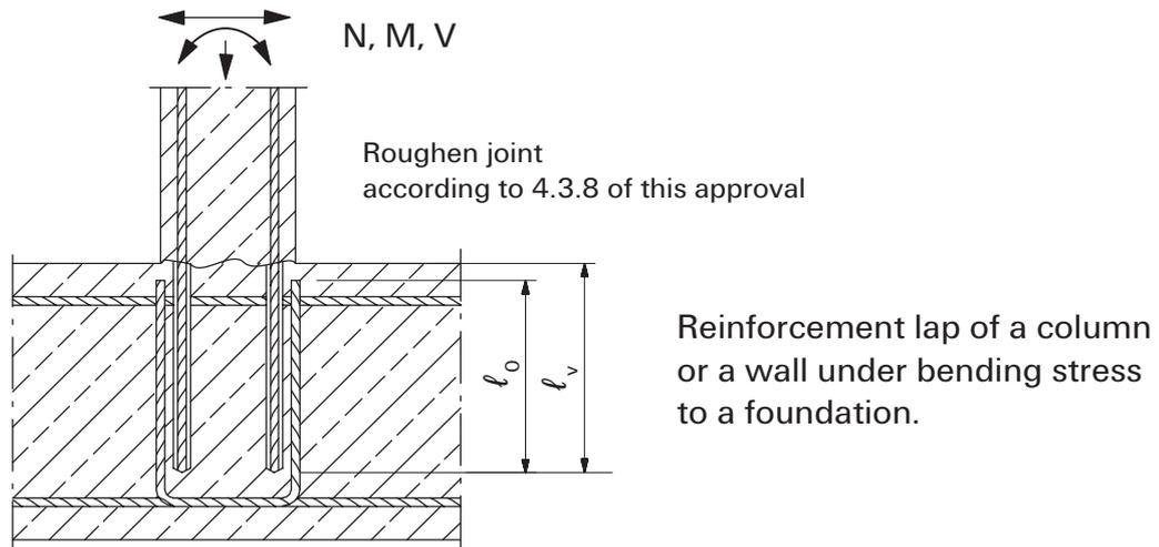
The required transverse reinforcement according to EN 1992-1-1 is not shown in the figures.
