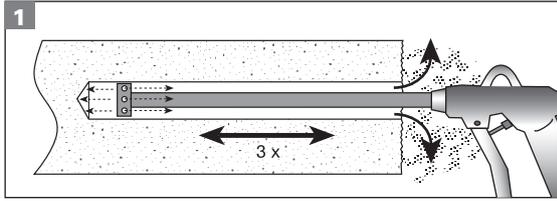
**Blowing out the drill hole**
