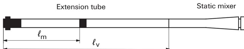
$l_v$  planned setting depth = drill hole depth = minimum length of the extension tube
