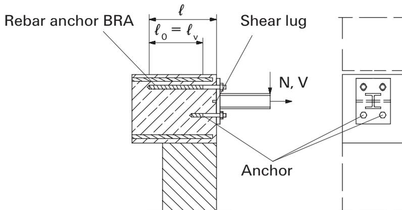
Lap of the anchoring of cantilevered building components
