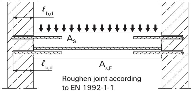
End anchoring of slabs or beams which have been designed as simply supported
