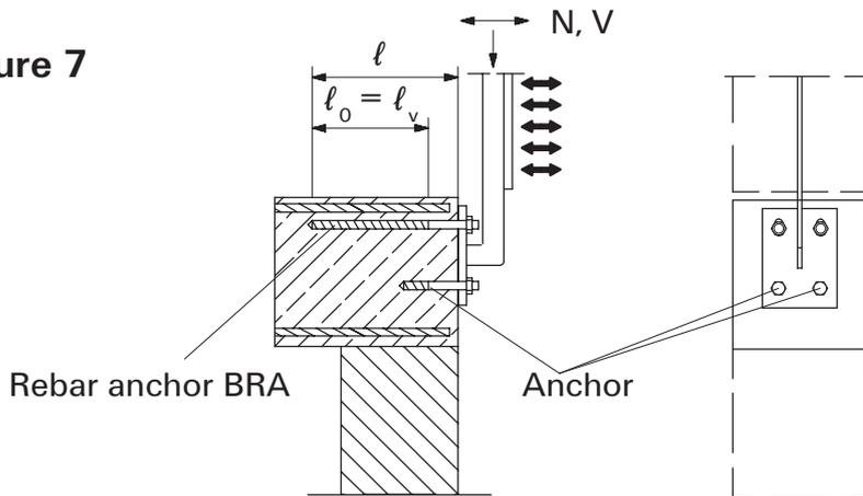
Lap for the anchoring of guardrail posts
