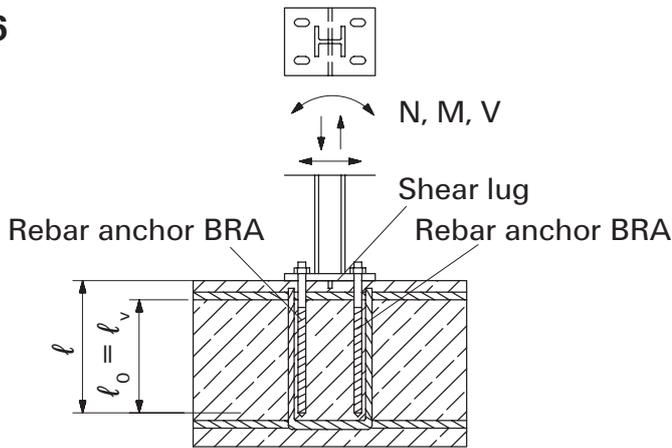
Lap to a foundation of a column under bending
