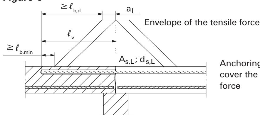
Anchoring of reinforcement to cover the envelope of the tensile force
