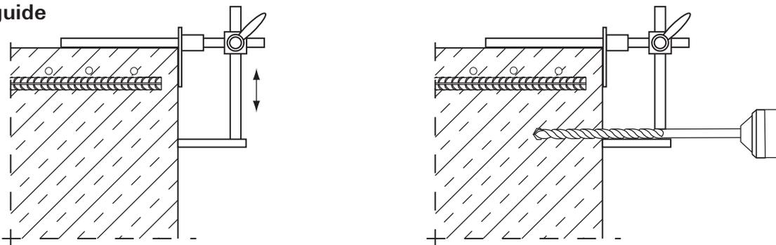
Rebar connection with Injection mortar MCS Uni Plus
