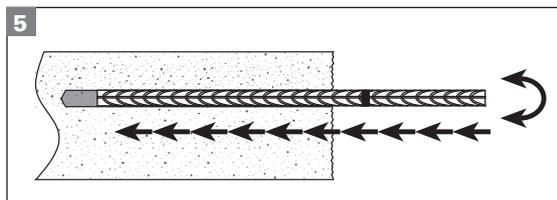
**Inserting reinforcement bar**
