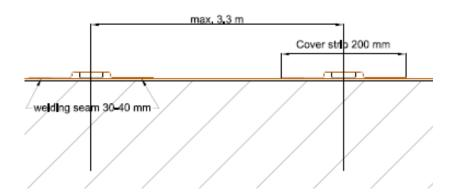
Minimum fastener distance $\geq 25 \text{ mm}$ Maximum fastener distance $\leq 500 \text{ mm}$ Minimum number of fastener2 piece/m²Maximum distance between fastener and edge of sheet $\geq 20 \text{ mm}$
