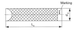
Marking: anchor size e.g.: M10 Stainless steel additional A4 e.g.: M10 A4 High corrosion-resistant steel additional C e.g.: M10 C
