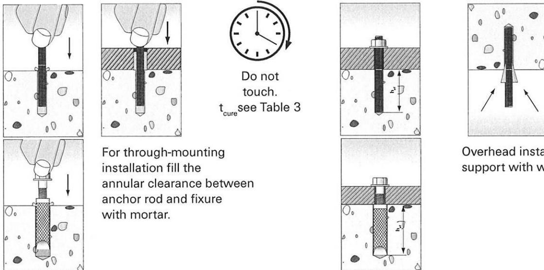
4) Insert the threaded rod MCS Plus A or internal treaded anchor MCS Plus I by hand using light turning motions until it reaches the setting depth marking. Excess mortar must exit the drill hole.
