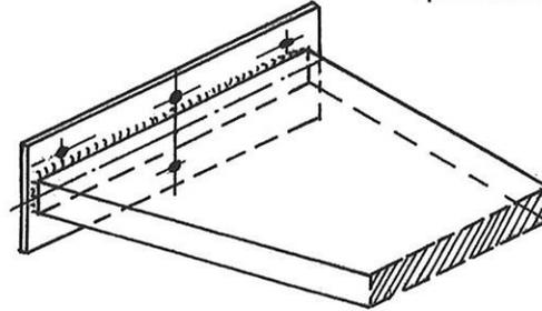
**Fastening to a cast-in steel stringer <sup>1)</sup>**
