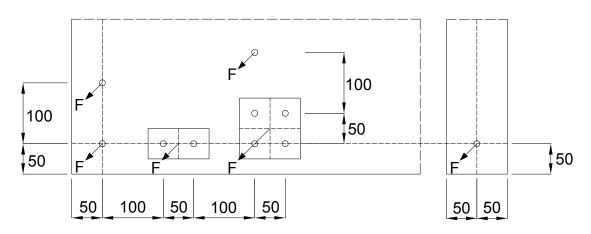
The characteristic resistance  $F_{Rk}$  applies to one fixing point. A fixing point can be:
