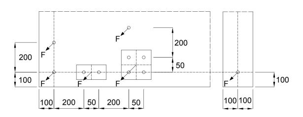
The characteristic resistance  $\mathsf{F}_{\mathsf{Rk}}$  applies to one fixing point. A fixing point can be:
