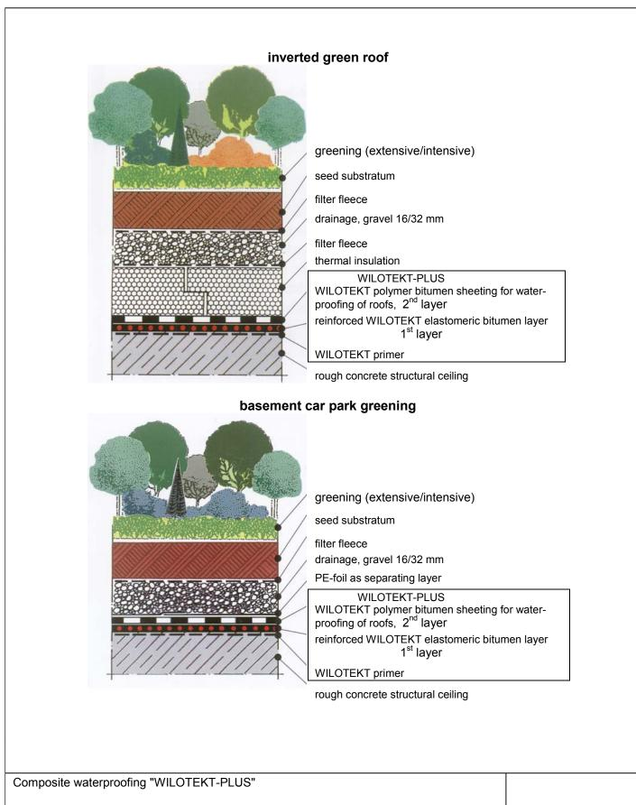
Possible applications of the composite waterproofing "WILOTEKT-PLUS"
